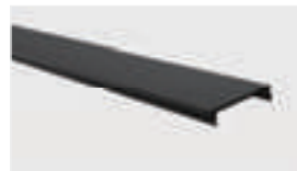
Track bind cover Model: CV-M20FB Material: PC Size: L1000*W25.7*H5.6mm Applicable model: All straight track
